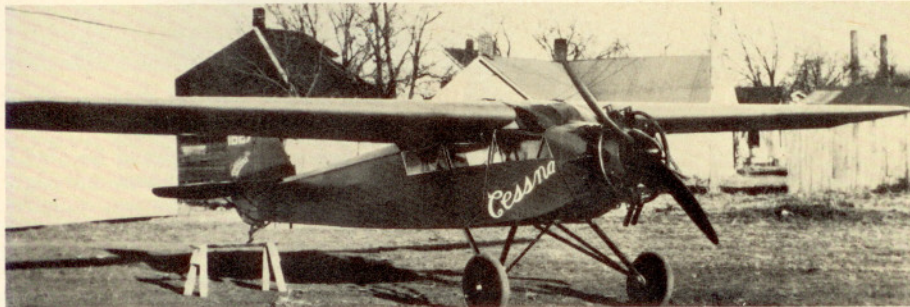
The original Cessna in its fourth configuration—with modified cabin and 120 h.p. Anzani engine that made it prototype of the Cessna "A" series. Registration number, X-1627, was later changed to 4165.
