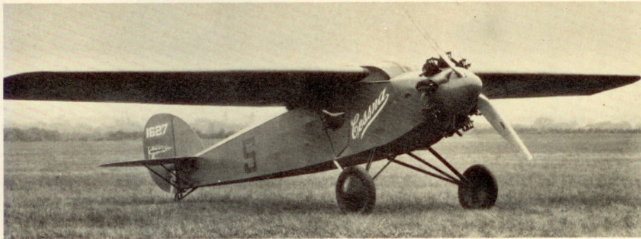
The 1927 Cessna modified for racing, with a 200 h.p. Wright J-4 engine and an enclosed cockpit. This was modified further to become pre-production prototype of the Cessna "B" model.
